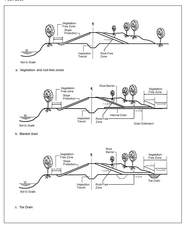
Figure 2-1. Basic levee project structure, with landscape planting
