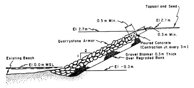
Figure 5-3. Quarrystone revetment
