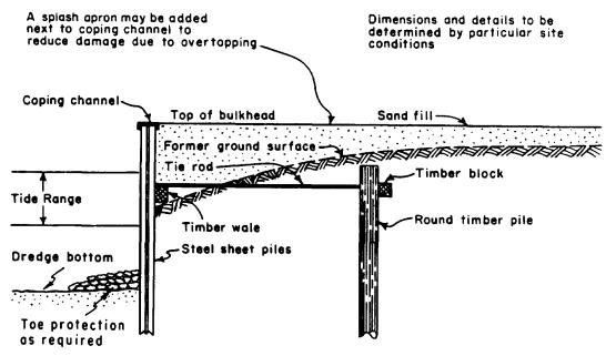
Figure 5-1. Steel sheet pile bulkhead
