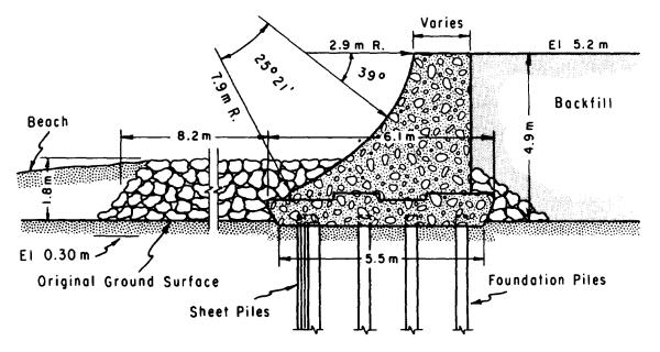
Figure 5-2. Concrete curved-face seawall
