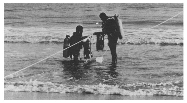
Figure 7-4. Diver using transect line in the surf
