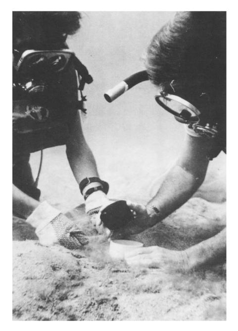
Figure 7-3. Core sampling at sandy-bottom stations
