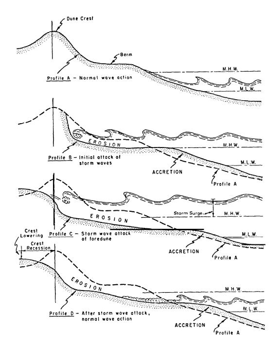
Figure 4-3. Schematic diagram of storm wave attack on beach and dune
