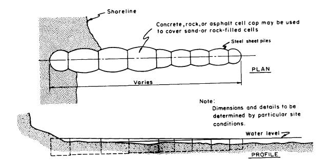
Figure 5-11. Irregular beach formed by cellular steel sheet-pile groin
