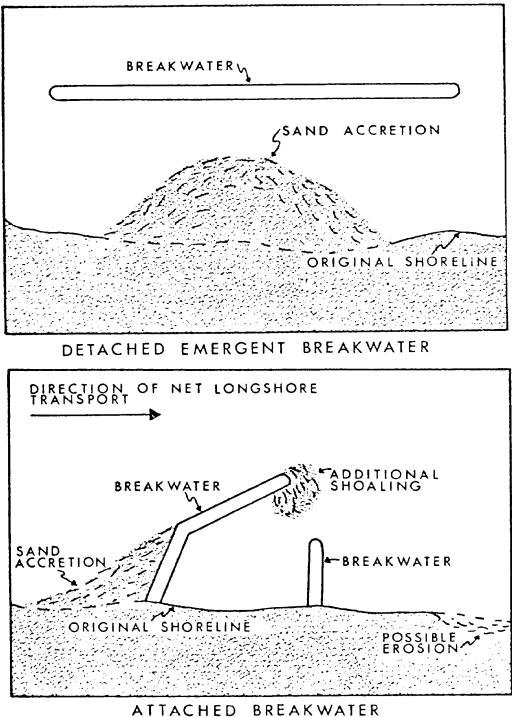
Figure 5-7. Erosion and accretion patterns in association with detached and attached breakwaters
